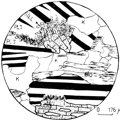
Şekil 6- Disten/Plajiolklas dokanağında yer alan sillimanitler, + N, DİS: Dişten, BİO: Biotit, K: Kuvars, PLJ: Plajiolklas, SİL: Sillimanit. Figure 6. Sillimanite needles at boundary between kyanite and plagioclase grains- + N, DİS: Kyanite, BİO: Biotite, K: Quartz, PLJ: Plagioclase, SİL: Sillimanite.
